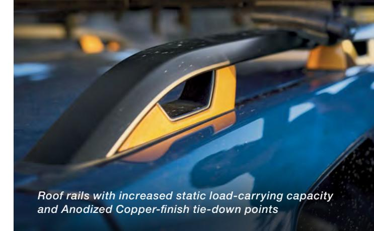
Roof rails with increased static load-carrying capacity
